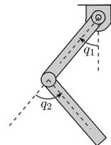
Fig. 1. The acrobot is a two-link articulated robot actuated only at the joint connecting the two links and thus underactuated. It resembles a gymnast swing on a high bar.
