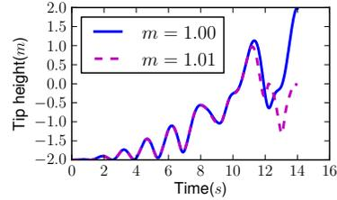
Fig. 2. The acrobot dynamics is sensitive to model parameters. With the same open-loop policy, the acrobot may succeed or fail, as a result of 1% difference in the model parameters.
